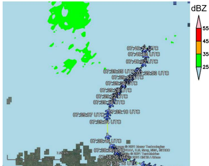
Figure 8: The superimposed accident flight profile based on ADS-B- with BMKG radar weather image at 1438 LT
